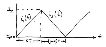
$V_s = 600$  V,  $R = 0.25~\Omega,\, L = 20$  mH, E = 150 V, k = 0.1 to 0.9 and f = 250 Hz
